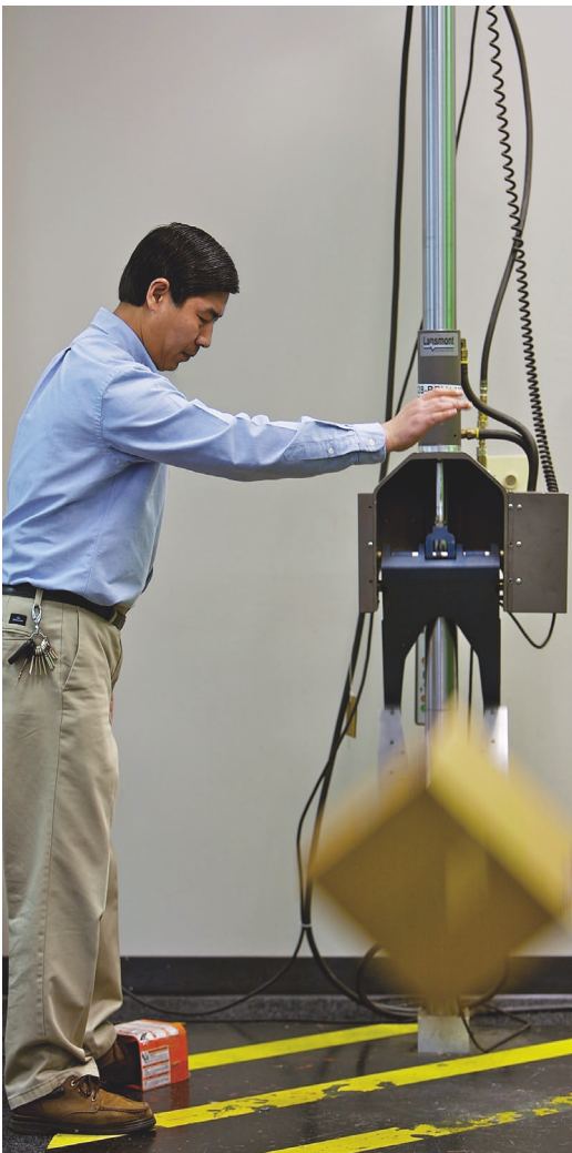
Lab engineer Yongquan Zhou performs a drop test on a package to determine how well it can withstand shock.
