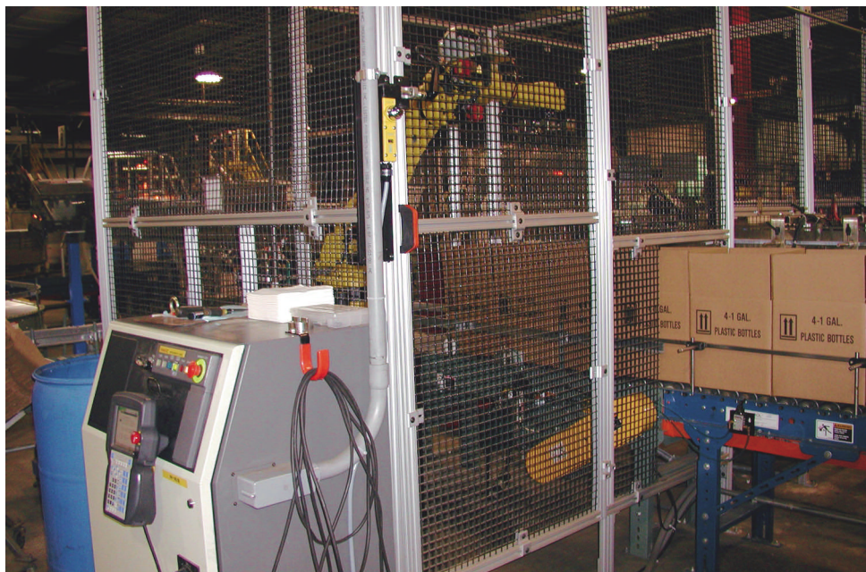
Running two shifts a day, five days a week, the robot (behind the safety fencing) fits into a tight space where the earlier manual packing was performed. Cage doors require special key access.
