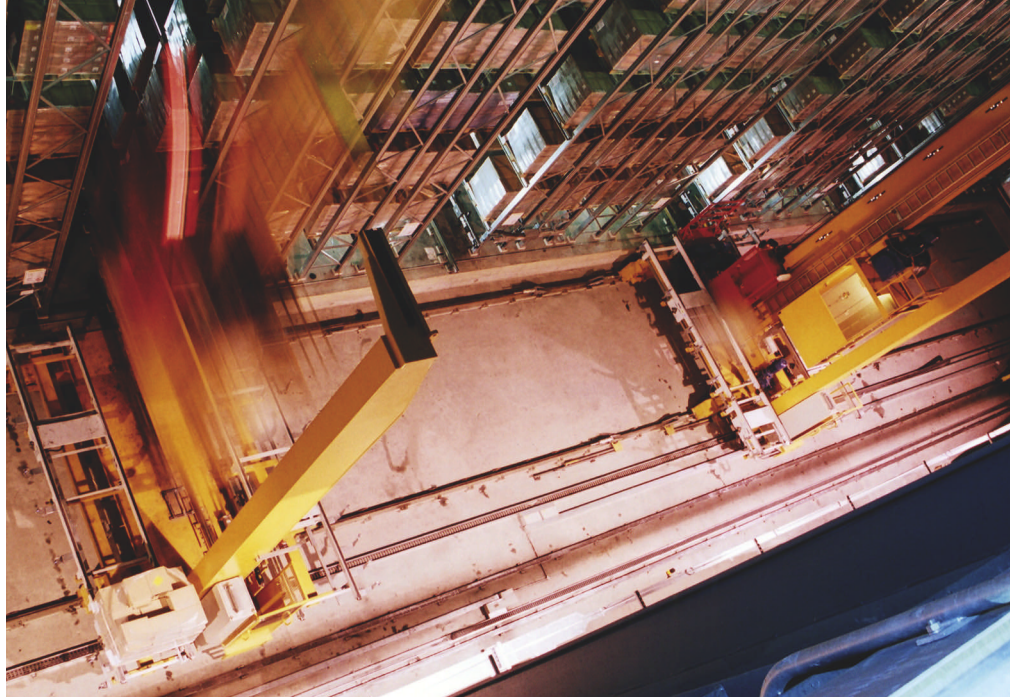
Two of the 17 storage-and-retrieval cranes in the finished-goods store, which has more than 12,000 pallet-storage locations.
