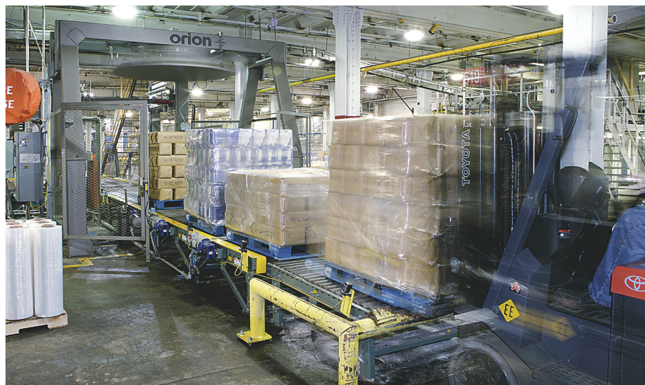
Pallets, above left, are automatically top-sheeted by a new dispenser before being shrink-wrapped to protect them from dust or contaminants. One of the three new, tower rotary stretch wrappers that carry out the main wrapping functions, above right, can wrap up to 120 loads/hr. The new systems complete in two shifts what formerly took three shifts.
