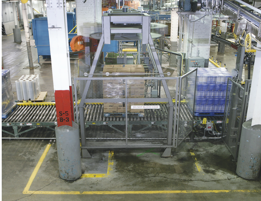
A pallet load enters the work zone, above, and the wrapping cycle begins. The wrappers are on what American Sugar Refining calls a 'main highway' of travel in the plant.
