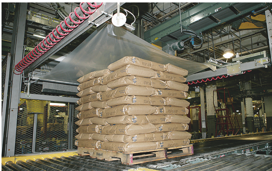
Pallets, above left, are automatically top-sheeted by a new dispenser before being shrink-wrapped to protect them from dust or contaminants. One of the three new, tower rotary stretch wrappers that carry out the main wrapping functions, above right, can wrap up to 120 loads/hr. The new systems complete in two shifts what formerly took three shifts.
